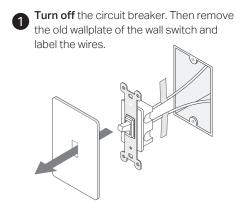
Ground: Usually green or copper. Neutral: Usually white, not connected to the dumb switch. Line/Load: Usually black, and connected to the dumb switch.
